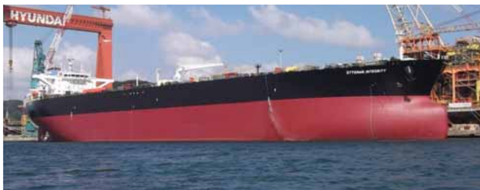
The first of the two super efficient Suezmaxes seen fitting out.
