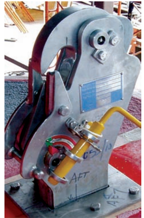
SeaCure lifeboat release and retrieval system.
