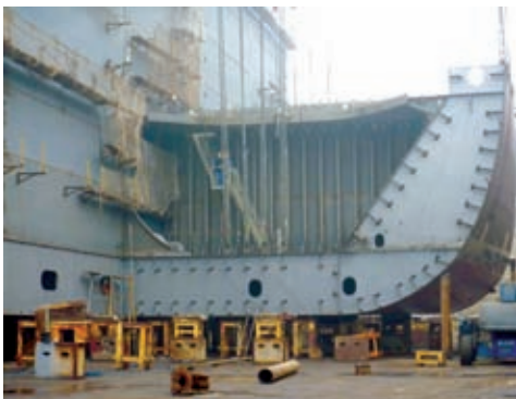
The forward end blocks of OSG's first VLCC to be constructed in China, which will be named Overseas McKinley when launched at DSIC Dalian Shipyard.
