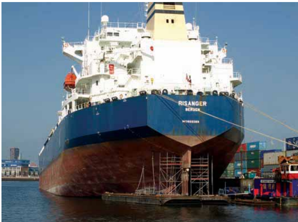
Risanger was ballasted down by the head to lift the stern, thus enabling afloat repairs to be undertaken.
