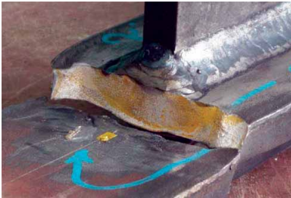
An example of steel fatigue failure after experimental testing at low temperatures.
