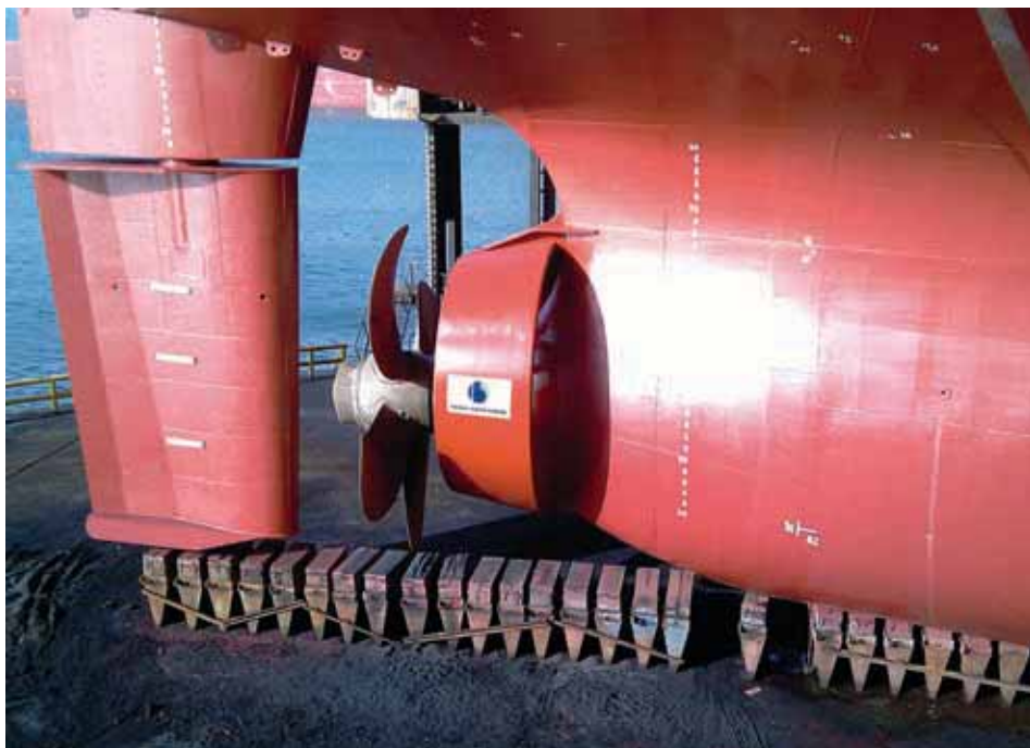
A single screw vessel fitted with a Becker Schilling rudder.
